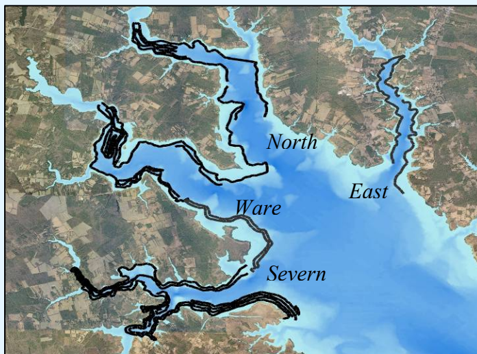
Figure 2. Acoustic survey tracklines
