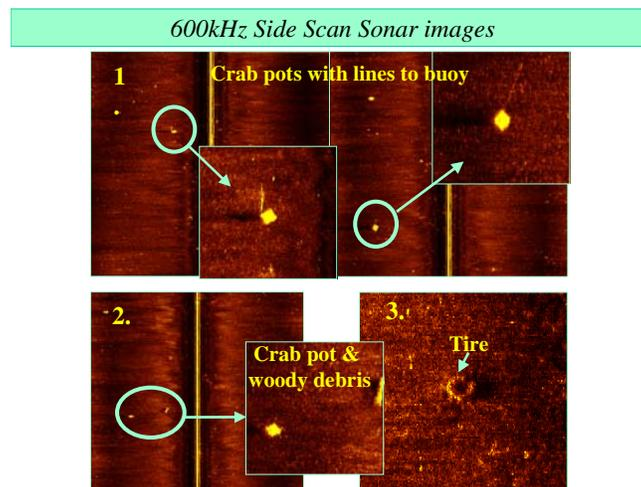
Figure 1. Side-scan image of derelict blue crab traps.
